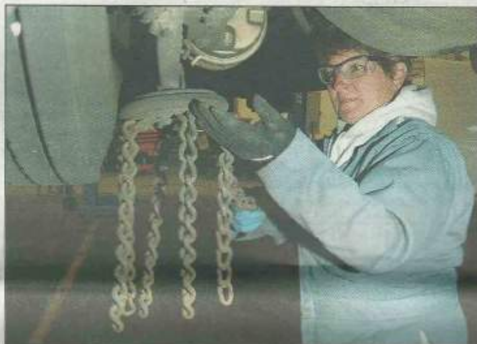
Peninsula School District mechanic Joni Gupille inspects one of the many school bus Onspot automatic snow chain systems.
